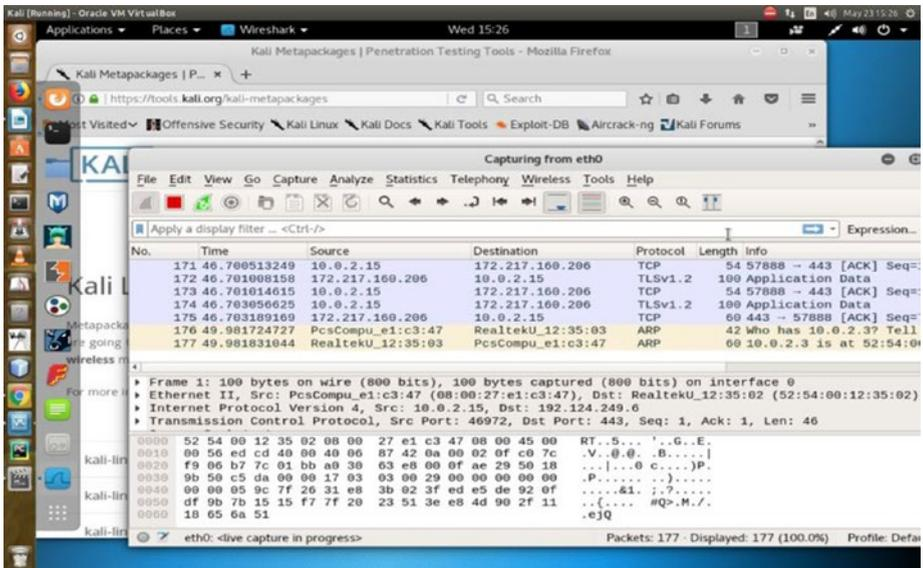
**Figure 9-2.** Wireshark is running and capturing traffic
