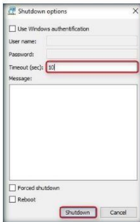
FIGURE 2.11: Shutting down a virtual machine remotely
