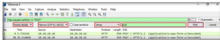
FIGURE 3.13: Wireshark - Selecting Options in Find Packet Window
