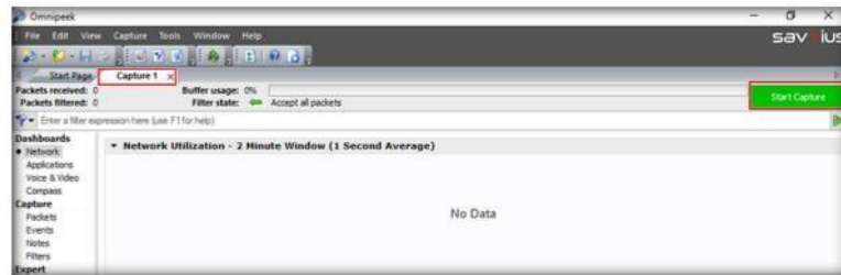
FIGURE 5.17: Starting packet capture
