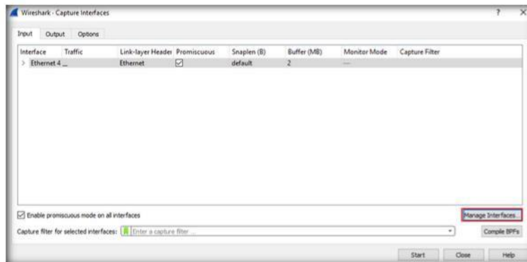
FIGURE 3.28: Selecting Options from Wireshark
