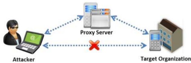
FIGURE 3.8: Attacker using a proxy server for connecting to the target
