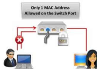
FIGURE 8.13: Blocking MAC Flooding
