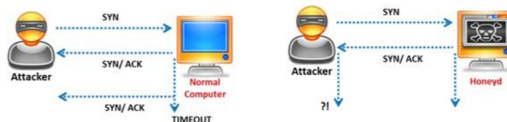
FIGURE 12.8: Response to SYN request by normal computer vs. Honeyd Honey pot
