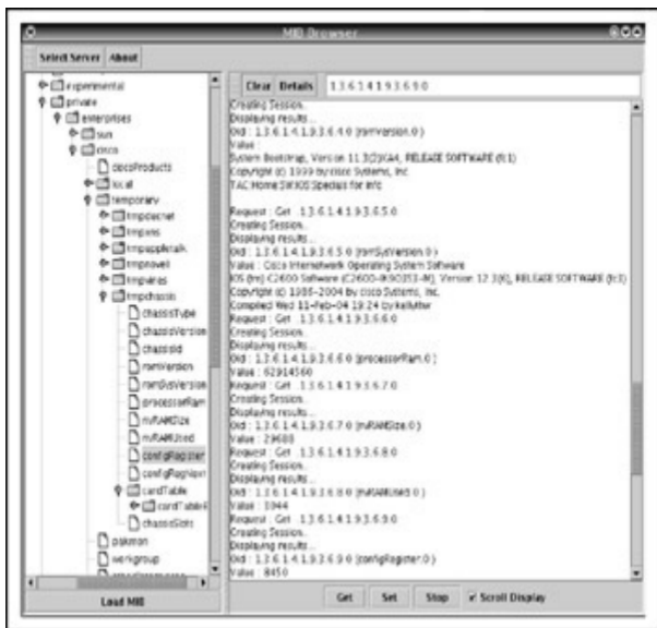
Figure 6-13: DwMibBrowser, looking at a Cisco 2600 router
