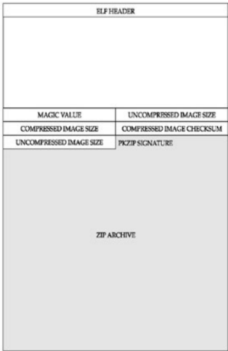
Figure 10-5: A structure of the self-extractable IOS image file
