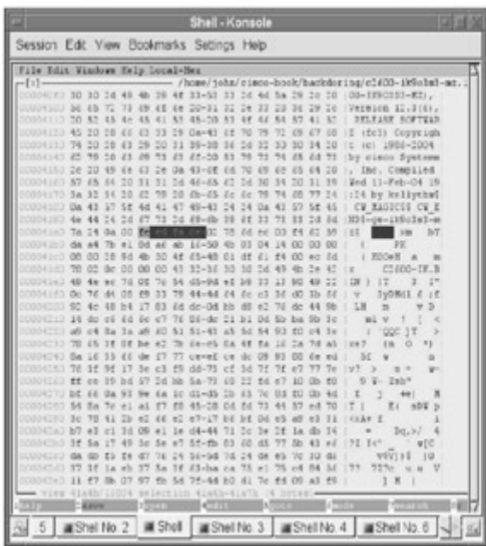
Figure 10-4: Magic v value in the IOS header
