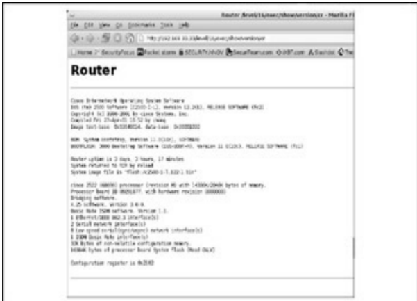
Figure 7-11: This Cisco device is vulnerable to arbitrary administrative access vulnerability.
