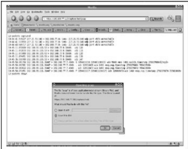
Figure 10-1: Viewing and downloading captured traffic from a PIX firewall
