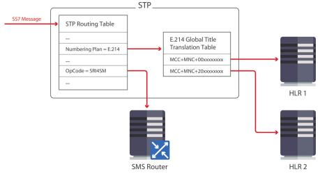
Figure 1 STP Routing misconfiguration.
