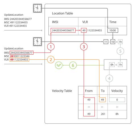
Figure 4 SS7 firewall bypass.
