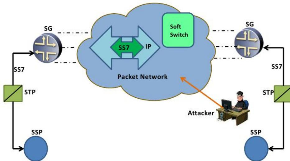
Figure 4.1: SS7 over IP (SIGTRAN) Experimentation Setup
