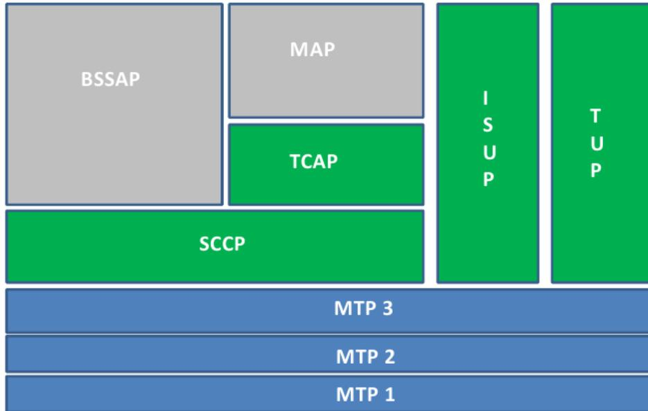
Figure 2.5: SS7 Protocol Stack for the GSM Network System [44]
