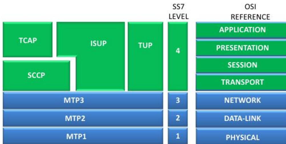
Figure 2.4: PSTN Based SS7 Protocol Stack [47]
