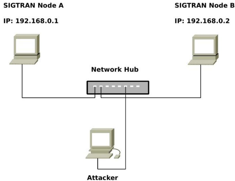
Figure 4.2: SIGTRAN Simulation Experimental Setup
