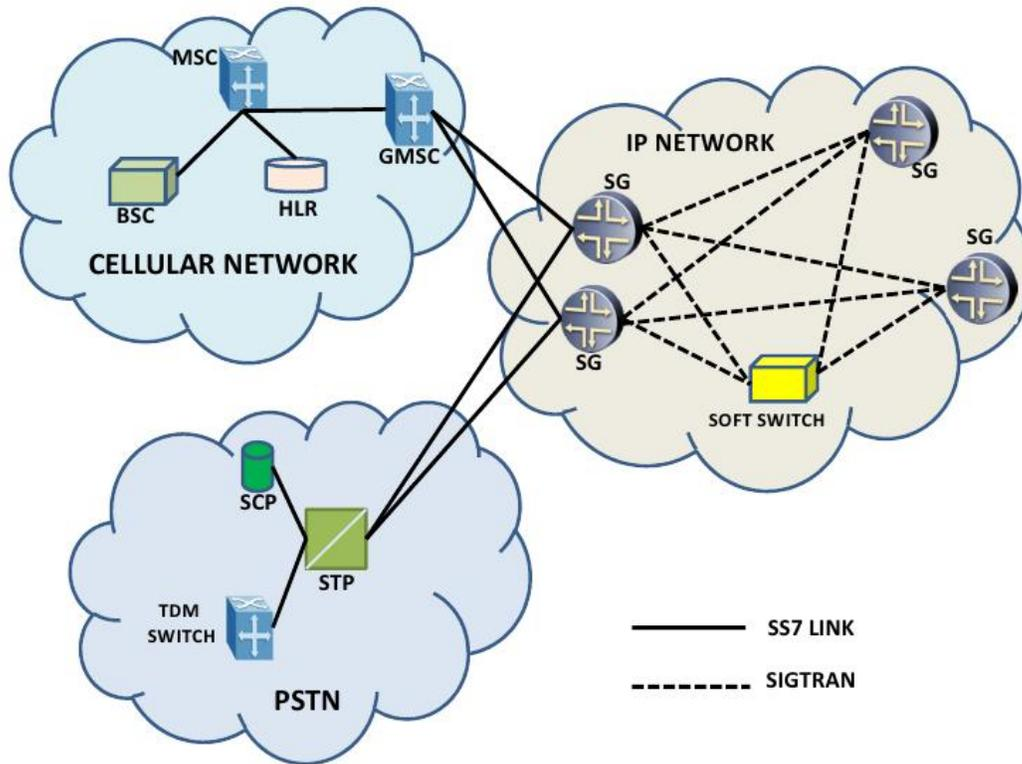
Figure 2.10: Internetwork Signaling Connection Using Signaling Gateway [36]
