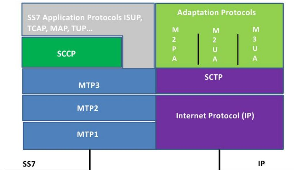
Figure 2.7: SIGTRAN Interface Protocol Stack [48]
