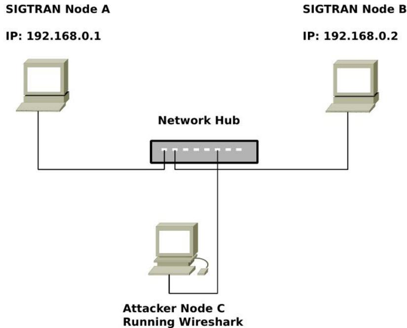
Figure 5.1: Network Sniffing Experiment Setup
