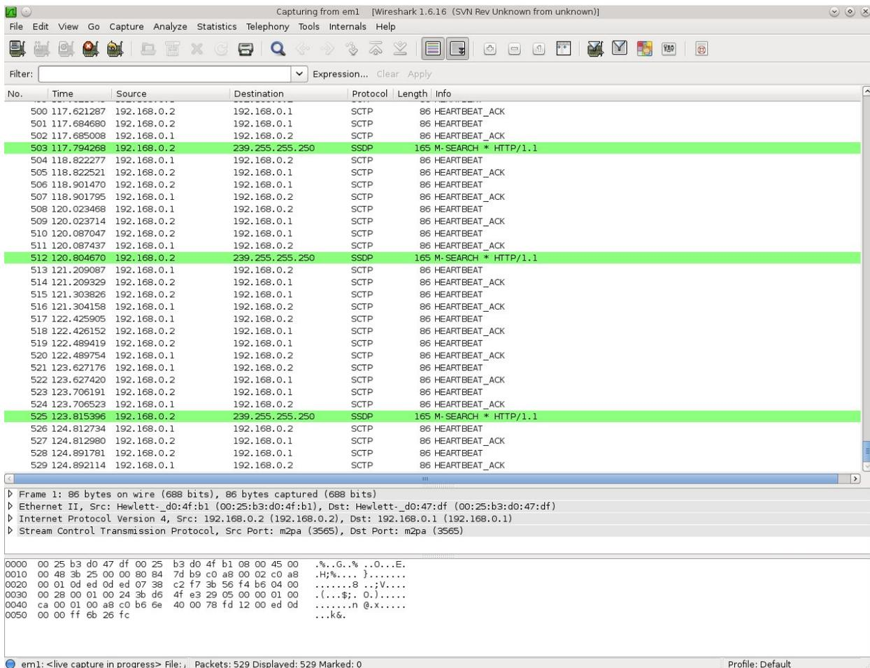
Figure A.1: Screenshot of Wireshark Network IP Capture
