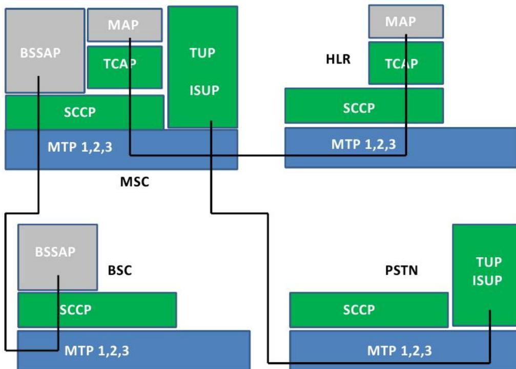
Figure 2.6: SS7 Protocols in Different Network Elements [44]
