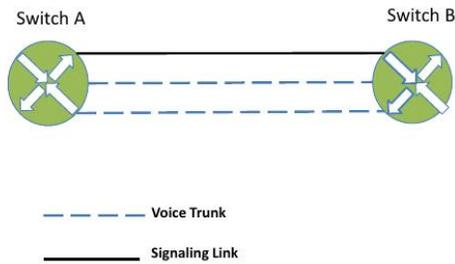
Figure 2.1: Channel Associated Signaling [46]
